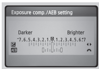
Canon Rebel T2i/550D LCD showing AEB with \pm 2 EV increments selected
