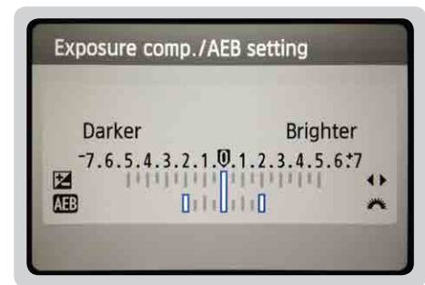
Canon Rebel T2i/550D LCD showing AEB with \pm 2 EV increments selected
