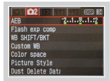
Canon Rebel XT/400D LCD showing AEB with \pm 2 increments selected
